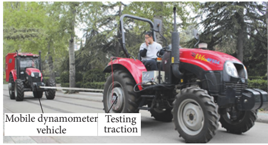
FIGURE 7: Traction test of YTO-MF554.
