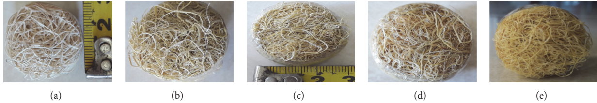
FIGURE 1: Photographs of the test panel sample. (a) Raw; (b) 1% NaOH; (c) 2% NaOH; (d) 5% NaOH; and (e) 8% NaOH.
