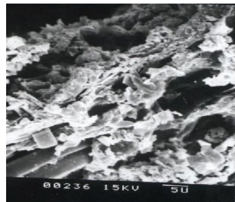
FIGURE 6: Membrane section of 30°C coated fertiliser (×2000).
