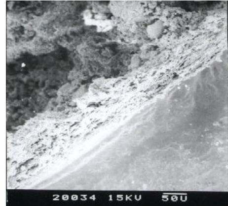
FIGURE 4: Section of 30°C coated fertiliser (×200).
