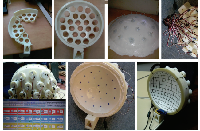
FIGURE 3: The early printed model of the dynamic subreflector. It was mostly printed using a 3D-printer. Each position accommodated a round shape housing which simplified the assembly process.
