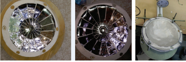
FIGURE 2: Several RF-reflecting materials were tested; they all had high reflecting results, but connecting them to the flexible surface was troublesome.
