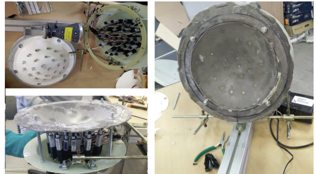
FIGURE 4: The advanced model of the dynamic subreflector. It was mostly made of complex materials, and each linear actuator was placed and locked to the surface allowing a tight structure while maintaining the flexibility of the dynamic RF membrane.
