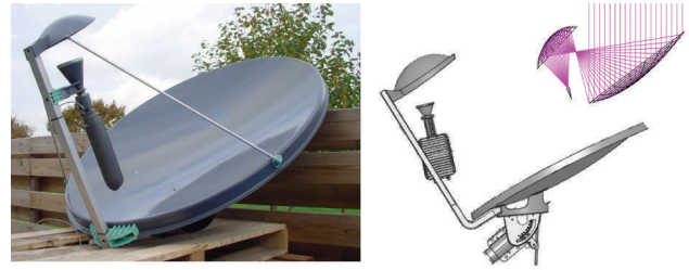
FIGURE 1: The general structure of a dual-reflector antenna. The static subreflector (shown on the upper part of the figure) was replaced with a dynamic surface mechanism.
