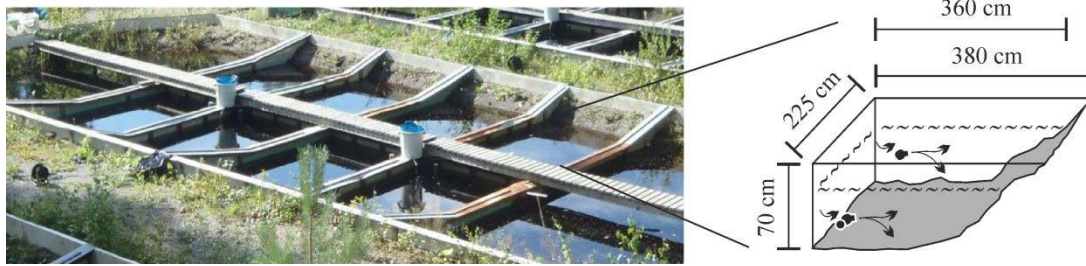
Fig. 2. Outdoor mesocosms used and a schematic presentation of one pond (IV). Three complexes including 12 ponds were employed in the experiments (one complex shown in the figure) using eight identical ponds in the middle of each complex, leading to a total number of 24 ponds. The wavy dashed line in the schematic presentation indicates the water table; the single arrows represent water inlets and the splitting arrows water outlets of the pumps.
