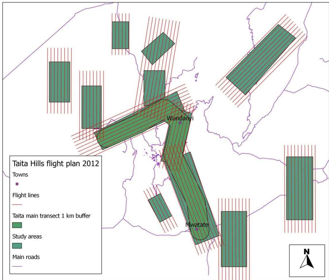
Figure 10. Flight plan for the flight campaign carried out in the Taita Hills in late January to early February in year 2012 (MosaicMill 2014). Taita main transect was covered for the CHIESA project. Other study areas marked with light green are used in other studies.
