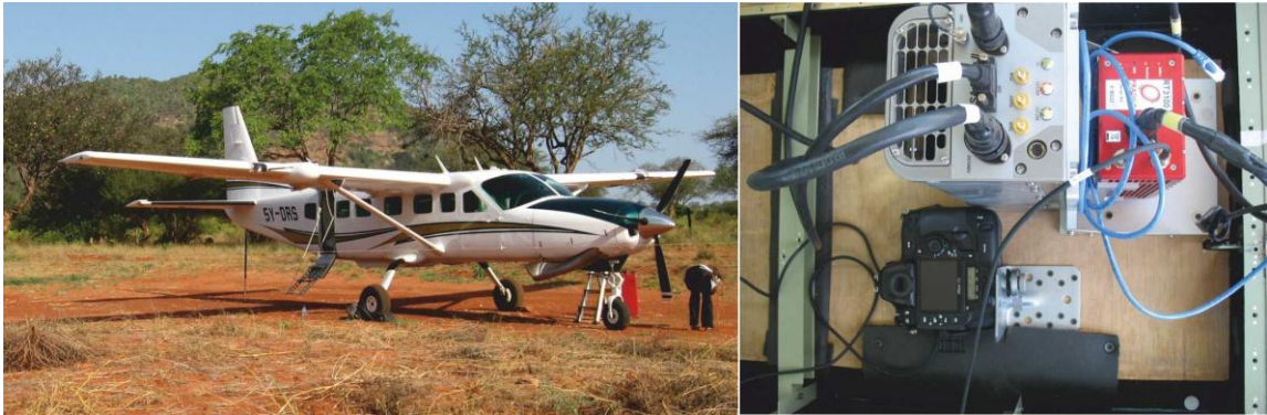
Figure 6. Cessna 208B Caravan I aircraft used in the campaign (left) and AisaEAGLE and Nikon D3X sensors mounted on the bottom of the aircraft. Images are taken by Tuure Takala and Pekka Hurskainen.
