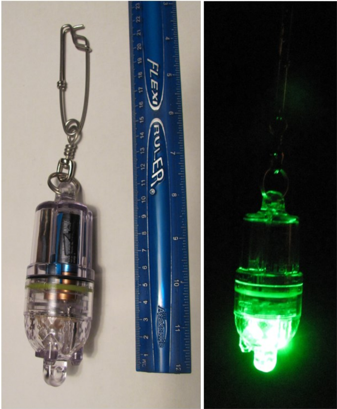
Figure 2.2 Photos of a battery powered artificial light that was hung vertically between fish pot entrances for pots undergoing light treatment. Both photos are of the same fishing light with the photo on the right taken in the dark.
