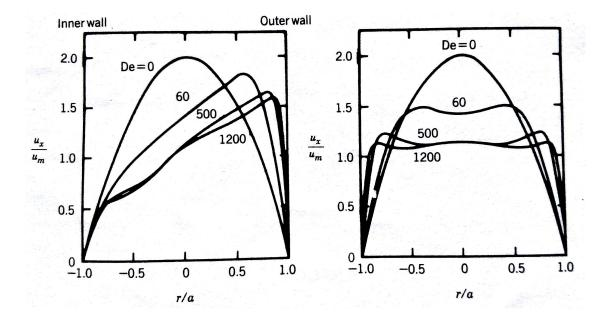
Figure 2.6: The influence of the Dean number on axial velocity profiles in a horizontal curved tube: (a) horizontal plane, (b) vertical plane [46]
