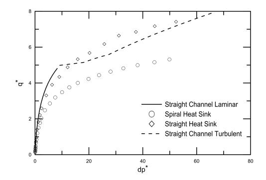
Figure 4.11: Dimensionless heat transfer versus dimensionless pressure drop comparison
