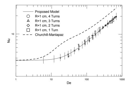
Figure 7.9: Model prediction for 1 cm curvature and 0.65 cSt oil
