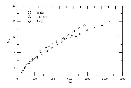
Figure 7.13: Viscosity effect on the curved tubing with three turns of 1 cm radius
