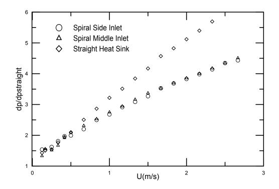
Figure 4.10: Pressure drop comparison of the heat sinks versus water velocity
