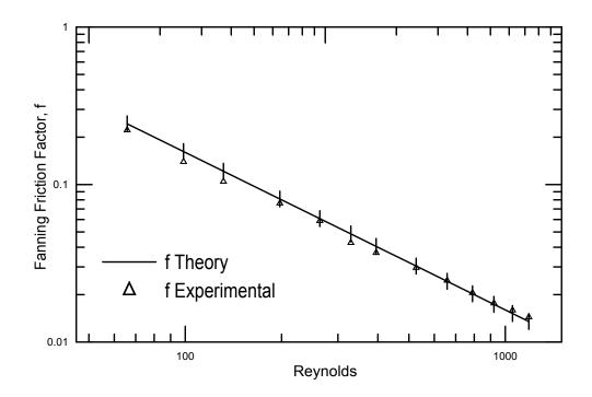
Figure 6.2: Benchmarking results for a straight tube, with error bars represent  $\pm 10\%$
