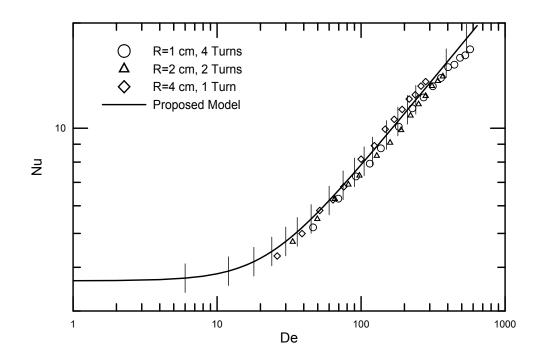
Figure 7.8: Proposed model prediction for constant length of 0.26 m and different curvatures with water
