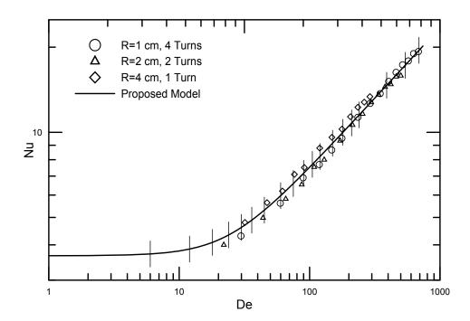
Figure 7.6: Proposed model prediction for constant length of 0.26 m and different curvatures with 0.65 cSt oil
