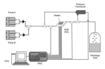
Figure A.2: Experiment configurations of the heat sinks tests
