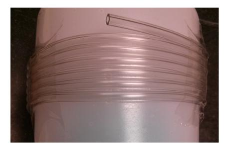
Figure A.5: A coiled tube used for the pressure drop tests
