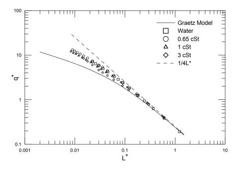
Figure 5.15: Viscosity effect on the curved tube with R = 8 cm and L = 25.12 cm
