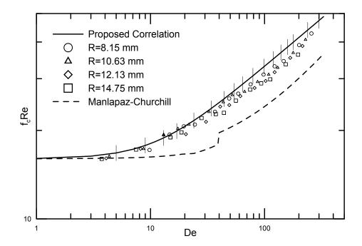
Figure 6.9:  $f_c Re$  vs De for 1.016 mm tube diameter and 0.5 m length
