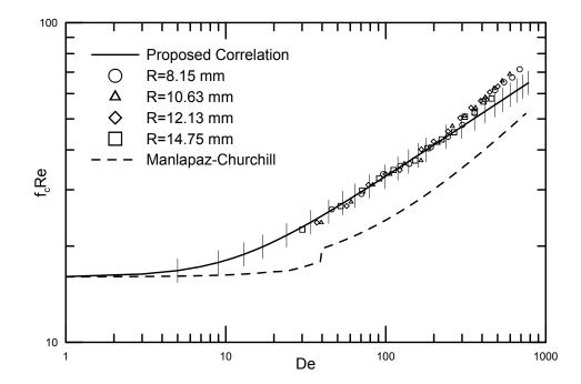
Figure 6.13:  $f_c Re$  vs De for 1.59 mm tube diameter and 0.5 m length
