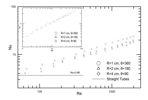
Figure 5.8: Nusselt analysis for different radius of curvature for water at L=6.28 cm
