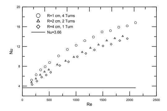
Figure 7.5: Heat transfer performance of different curvatures for constant length of 0.26 m with water
