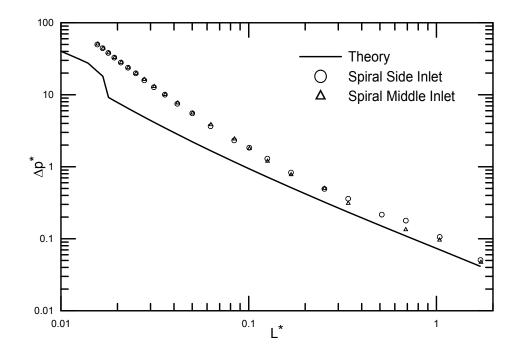
Figure 3.10: Pressure drop for the spiral channel with middle and side inlet comparison to the straight channel of an identical size
