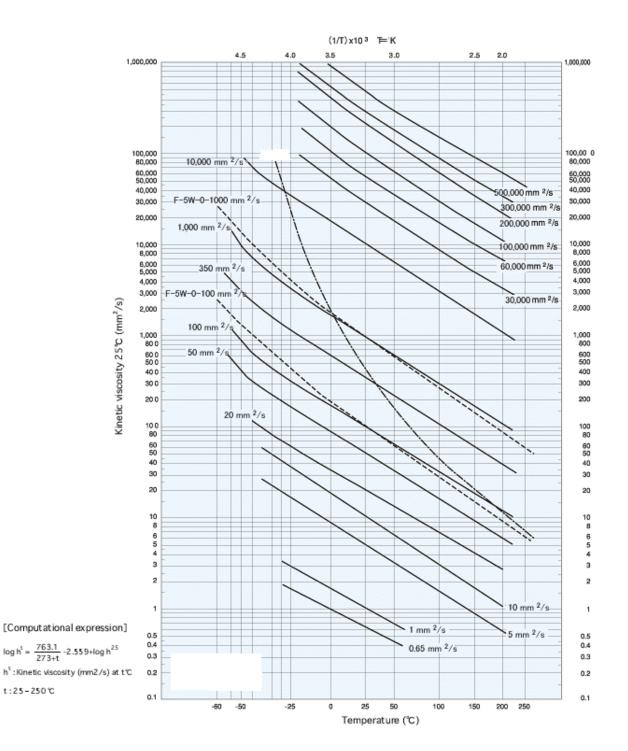
Figure A.9: Viscosity of the silicon Oils given by the company (Clear Co.)
