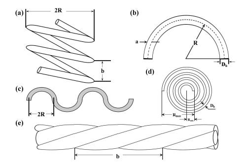
Figure 2.1: Different type of curved tube geometries: (a) helical coil, (b) bend tube, (c) serpentine rube, (d) spiral and (e) twisted tubes
