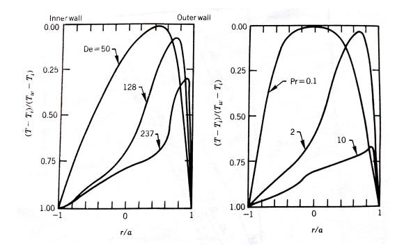
Figure 2.10: The dimensionless horizontal temperature profile for T boundary condition as a function of a) Dean number and b) Prandtl number for a curved tube
