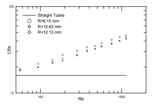
Figure 6.4:  $f_c Re$  vs Re for 1.27 mm tube diameter and 1 m length
