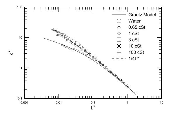
Figure 4.5: Different fluid performance for the side inlet spiral channel heat sink
