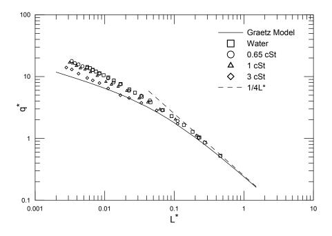
Figure 5.14: Viscosity effect on the curved tube with R=2 cm and L=9.42 cm
