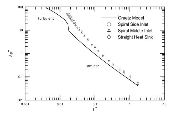
Figure 4.9: Dimensionless pressure drop comparison between the heat sinks
