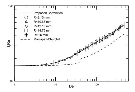
Figure 6.12:  $f_c Re$  vs De for 1.59 mm tube diameter and 1 m length
