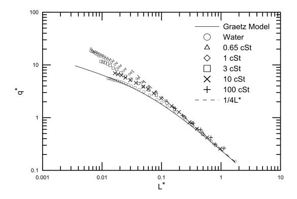
Figure 4.4: Different fluid performance for the middle inlet spiral channel heat sink
