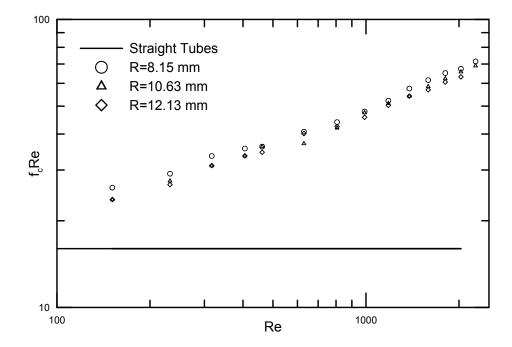
Figure 6.7:  $f_c Re$  vs Re for 1.59 mm tube diameter and 0.5 m length
