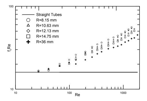
Figure 6.6:  $f_c Re$  vs Re for 1.59 mm tube diameter and 1 m length
