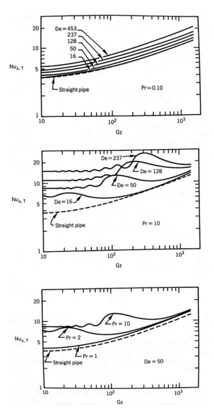
Figure 2.3: The influence of Prandtl number on the Nusselt numbers in the entrance region of a curved circular tube for the T boundary condition [46]
