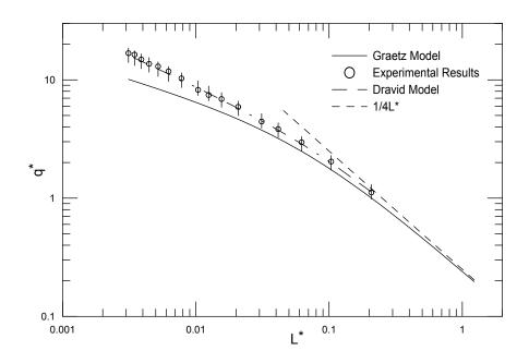
Figure 5.5: Dravid model comparison for 1 cSt silicone oil R=2 cm, L=9.42 cm with 10 percent error bars
