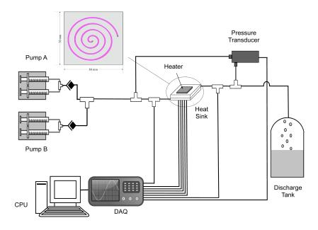
Figure 3.1: Experimental test setup and the spiral channel
