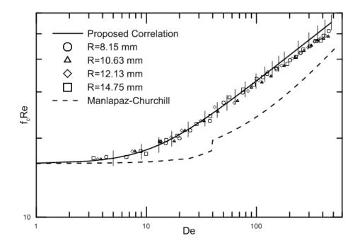
Figure 6.11:  $f_c Re$  vs De for 1.27 mm tube diameter and 0.5 m lengt
