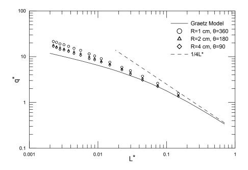
Figure 5.6: Different radius of curvature for water with L=6.28 cm
