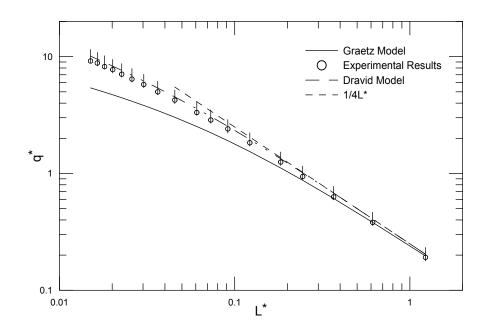
Figure 5.4: Dravid model comparison for the experimental results for water R=4 cm, L=25.12 cm with 10 percent error bars
