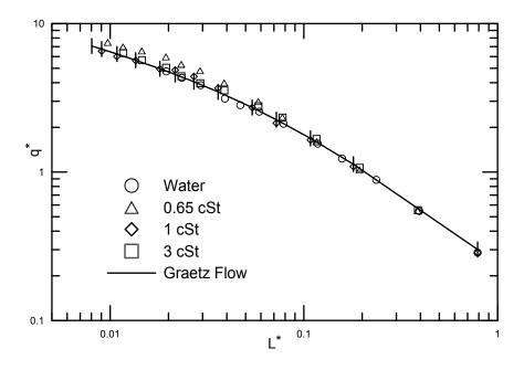
Figure A.7: Heat transfer benchmarking results for water and different silicone oils with 10% error bars
