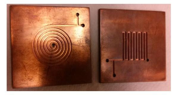
Figure 4.1: Spiral and straight heat sinks used in the experiments
