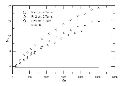
Figure 7.3: Heat transfer performance of different curvatures for constant length of 0.26 m with 0.65 cSt oil
