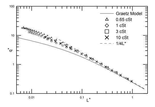
Figure 3.4: Different fluid performance for the side inlet spiral channel
