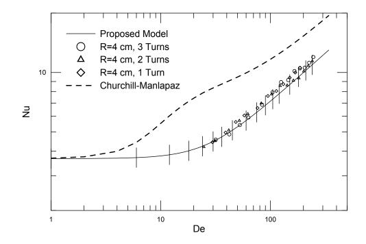
Figure 7.10: Model prediction for 4 cm curvature and 1 cSt oil
