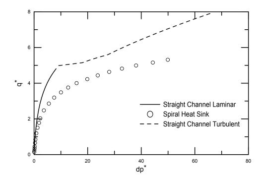
Figure 3.11: Pressure drop and heat transfer performance comparison of spiral channel and an identical straight channel
