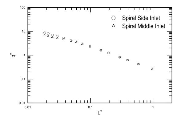
Figure 4.8: The entrance effect in the spiral heat sink for 10 cSt silicon oil
