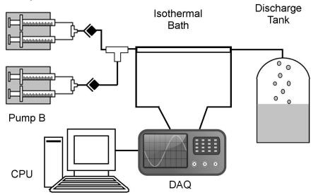
Figure 5.2: System configuration
