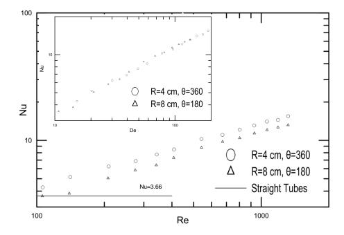
Figure 5.9: Nusselt analysis for different radius of curvature for 1 cSt silicone oil with L=25.12 cm
