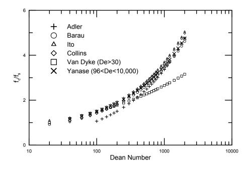
Figure 2.9: Numerical friction factor correlations comparison
