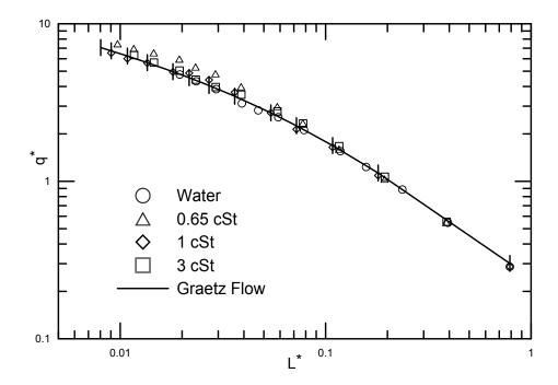
Figure 7.2: Benchmarking results for a straight tube, with error bars represent  $\pm 10\%$
