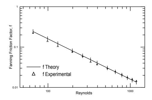
Figure A.8: Pressure drop benchmarking results for water with 10% error bars
