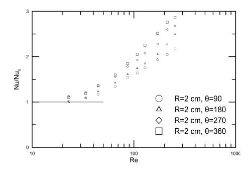
Figure 5.13: Normalized Reynold analysis for different lengths for 3 cSt silicone oil with R=2 cm
