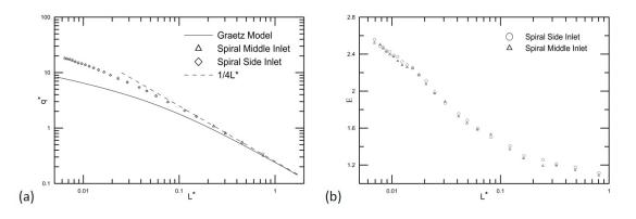
Figure 3.5: a) Inlet effect on heat transfer for 3 cSt silicone oil, b) Heat transfer enhancement ratio for 0.65 cSt silicone oil
