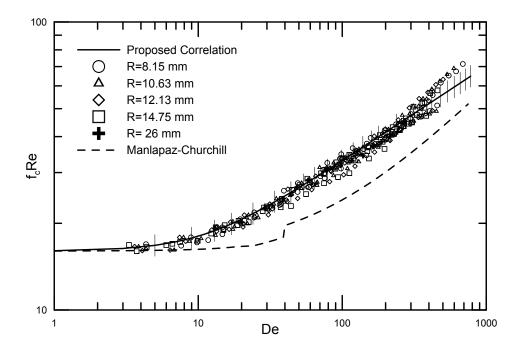
Figure 6.14:  $f_c Re$  vs De for all of the experimental results
