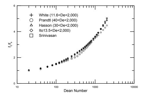
Figure 2.8: Experimental friction factor correlations comparison [33]
