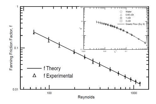
Figure 3.2: Pressure drop and heat transfer benchmarking test in straight circular tubes with 10% error bars
