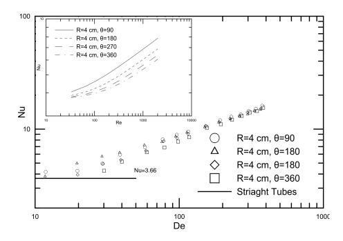
Figure 5.10: Nusselt analysis for different lengths for 0.65 cSt silicone oil with R=4 cm
