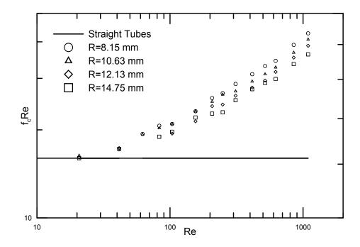
Figure 6.3:  $f_c Re$  vs Re for 1.016 mm tube diameter and 0.5 m length
