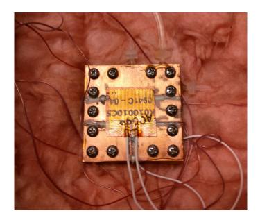
Figure A.3: A heat sink inside the insulation box
