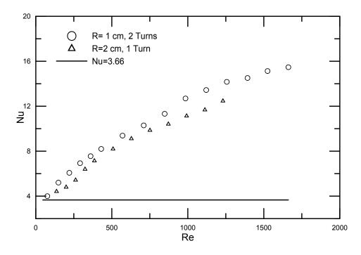
Figure 7.4: Heat transfer performance of different curvatures for constant length of 0.13 m with 1 cSt oil
