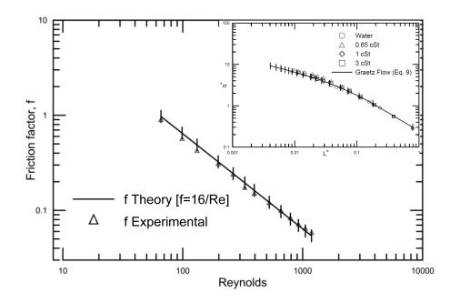
Figure 4.3: Pressure drop and heat transfer benchmarking test in straight circular tubes
