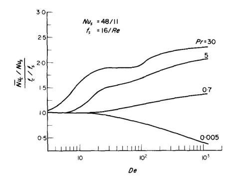
Figure 2.13: Effectiveness of curved circular tubes as compared to straight tubes [186]
