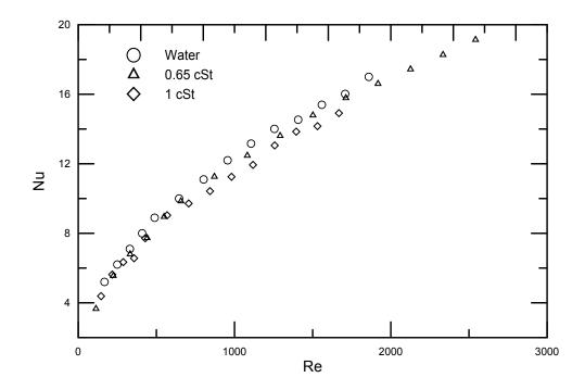
Figure 7.12: Viscosity effect on the curved tubing with three turns of 2 cm radius
