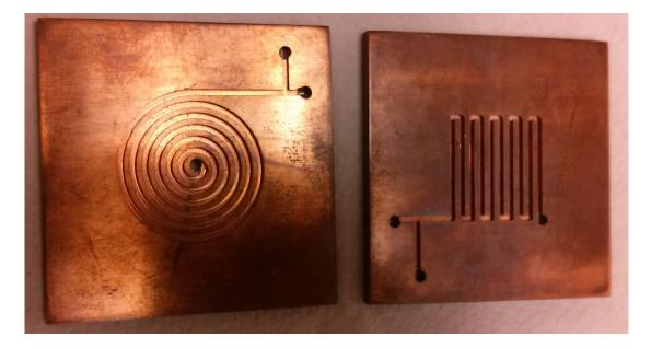
Figure A.1: Heat sinks channel patterns
