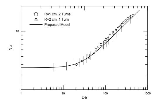
Figure 7.7: Proposed model prediction for constant length of 0.13 m and different curvatures with 1 cSt oil
