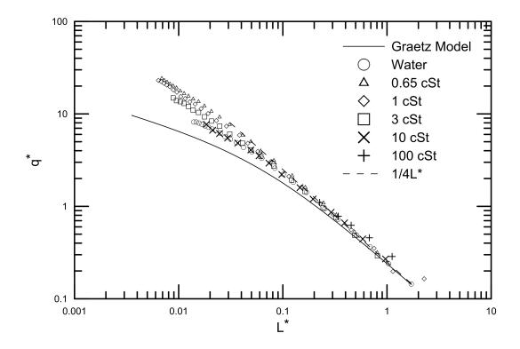
Figure 4.6: Different fluid performance for the straight channel heat sink
