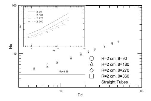
Figure 5.11: Nusselt analysis for different lengths for 3 cSt silicone oil with R=2 cm
