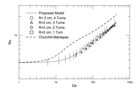
Figure 7.11: Model prediction for 2 cm curvature and water
