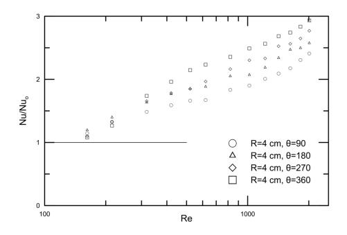
Figure 5.12: Normalized Reynolds analysis for different lengths for 0.65 cSt silicone oil with R=4 cm
