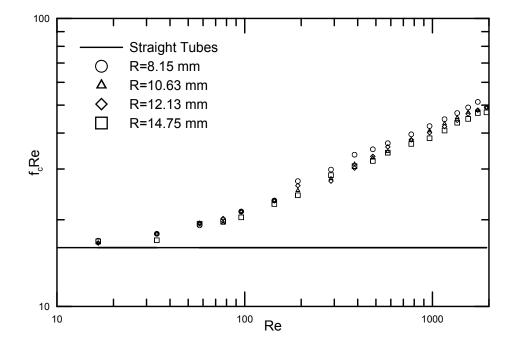
Figure 6.5:  $f_c Re$  vs Re for 1.27 mm tube diameter and 0.5 m length
