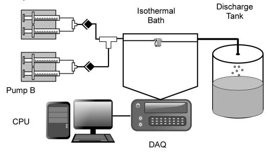
Figure 7.1: System configuration
