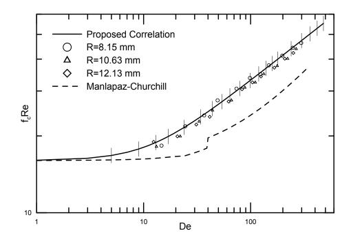
Figure 6.10:  $f_c Re$  vs De for 1.27 mm tube diameter and 1 m length
