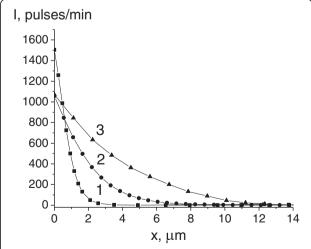
**Figure 1** Concentration distribution of the <sup>60</sup>Co radioisotope after 1, 50, and 200 cycles of transformation. Concentration distribution of the <sup>60</sup>Co radioisotope in reverted austenite after 1 (1), 50 (2), and 200 (3) cycles of transformation.
