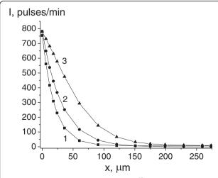
**Figure 2** Concentration distribution of the  $^{60}$ Co radioisotope after γ-ε-γ transformations and additional annealing. Concentration distribution of the  $^{60}$ Co radioisotope in reverted austenite after 1 (1), 100 (2) and 500 (3) cycles of transformation and additional annealing at 325°C.
