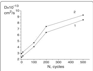
**Figure 3** The diffusion coefficient of cobalt change as a function of the number of γ-ε-γ cycles. The diffusion coefficient of cobalt change as a function of the number of γ-ε-γ cycles after diffusion annealing at 250°C (1) and 325°C (2).
