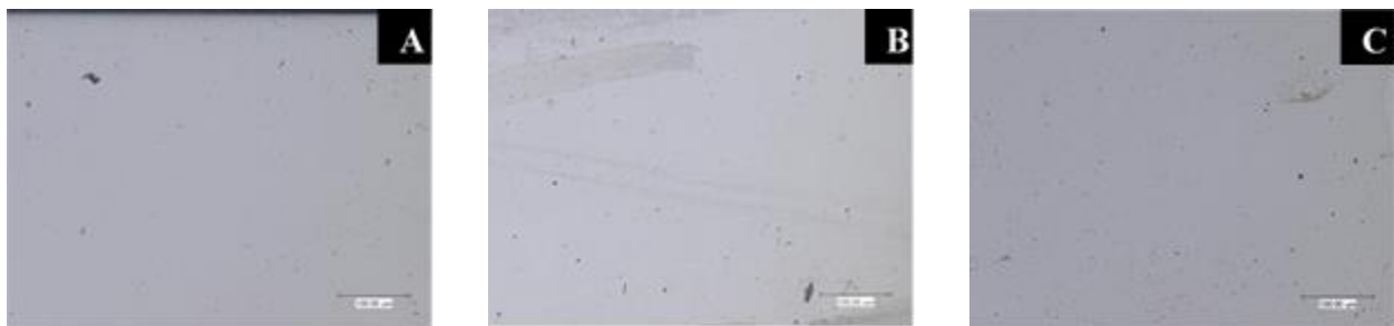
Figure 41. Micrographs of electrolytic etching of MPU alloy exposed for 22 hours (A), 220 hours (B), and 362 hours (C) at 700°C in dry air
