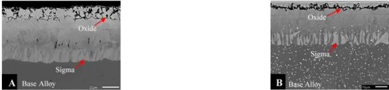
Figure 62. SEM BSE micrographs of MPS (A) and MEC (B) after 500 hour exposure at 700°C in a simulated anode environment
