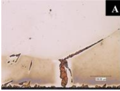
Figure 42. Micrographs of electrolytic etching of MPU alloy exposed for 500 hours at 700°C in dry air showing edge formation of sigma (A) and grain boundary formation of sigma (B)
