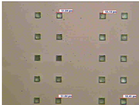
Fig. 7.11: Different sized holes used to test the Microflex technology
