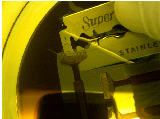
Fig. 7.27: Method of releasing the SPNI samples, after immersion in MIBK and IPA
