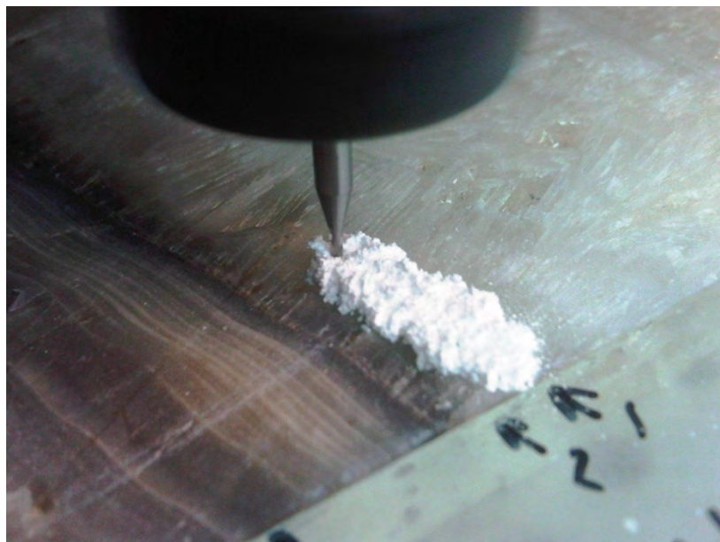
Figure S.12: Automated drilling of Yarrangobilly speleothem sample following growth laminations to maximise spatial resolution.
