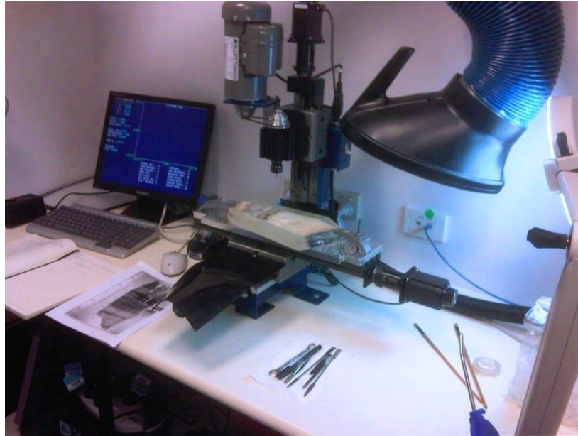
Figure S.13: Drilling stage setup and stage control interface.
