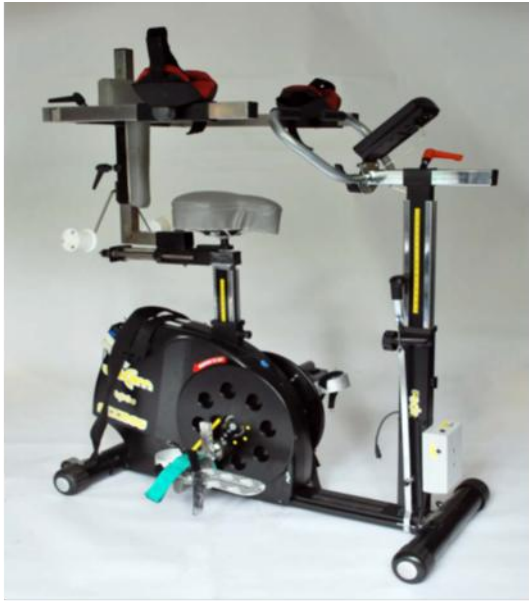
Figure 44. – The adapted cycle ergometer utilizing a body weight supporting saddle from Hancock (49)
