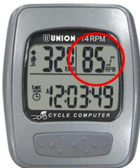
Figure 42. – Cycle computer. Digital read-out gives live feedback on cycling rpm (red circle)
