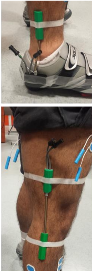
Figure 10. – Ankle (top) and Knee (bottom) goniometers placed over the respective joints to measure changes in position during cycling
