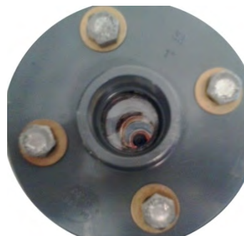
Figure 3.7 (c) picture of the PLIF rig;(d) window used to capture the cross section of glass pipe.
