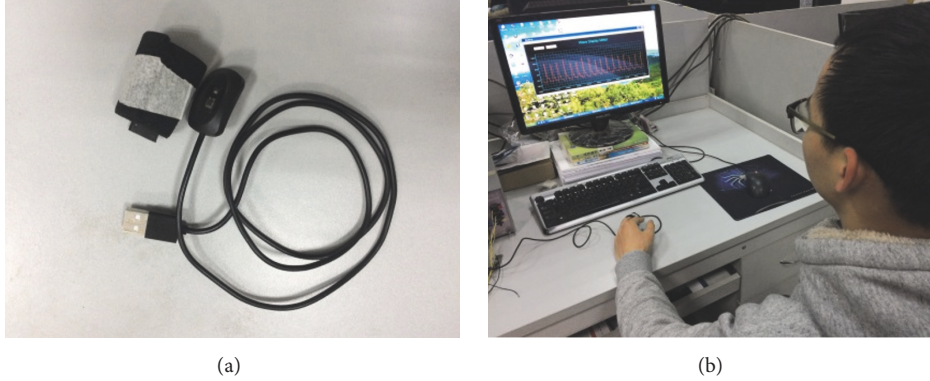
FIGURE 1: The monitoring scene using the reflective pulse oximeter. (a) The reflective pulse oximeter; (b) the PPG signals collection using the reflective pulse oximeter.
