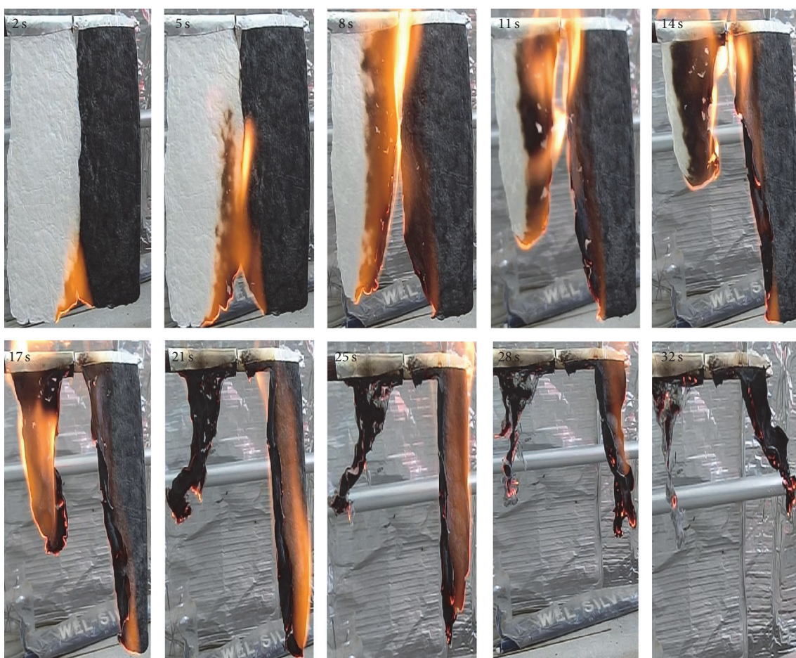
FIGURE 7: Photographs of flame retardancy test for the pure cellulose sheet (left white sample) and the CNT/cellulose sheet (right black sample). At t = 0 s, a fire is added on the bottom of the samples.
