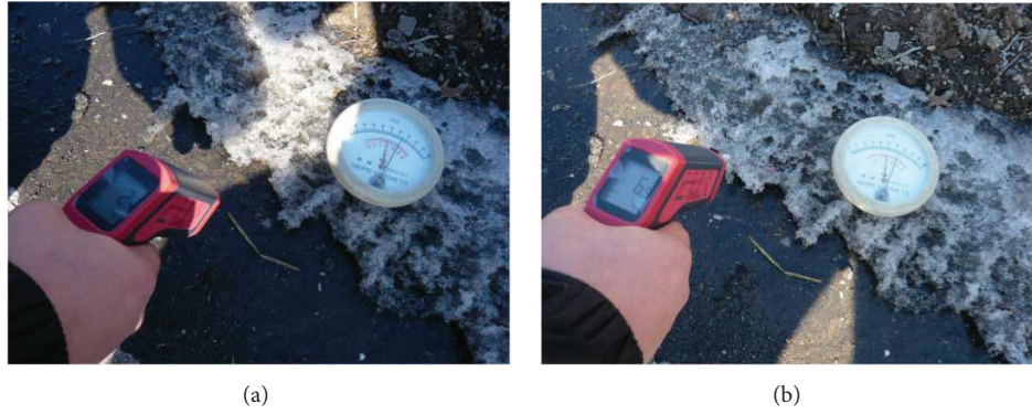
FIGURE 10: Temperature testing of the pavement outside the tunnel.
