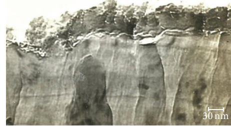
FIGURE 3: Transmission electron micrograph of ultramicrotomed section of the coating developed for 15 s on aluminium in a chromate bath.
