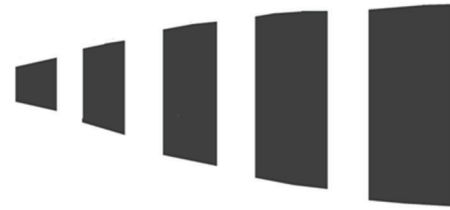
FIGURE 11: The rubber is cut according to the shape of the tail—the first 2 stripes from the tail fin (left on this picture are 20 mm wide and the remaining ones are 25 mm wide).
