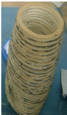
FIGURE 10: The rings were glued together to form the front part of the robot fish.
