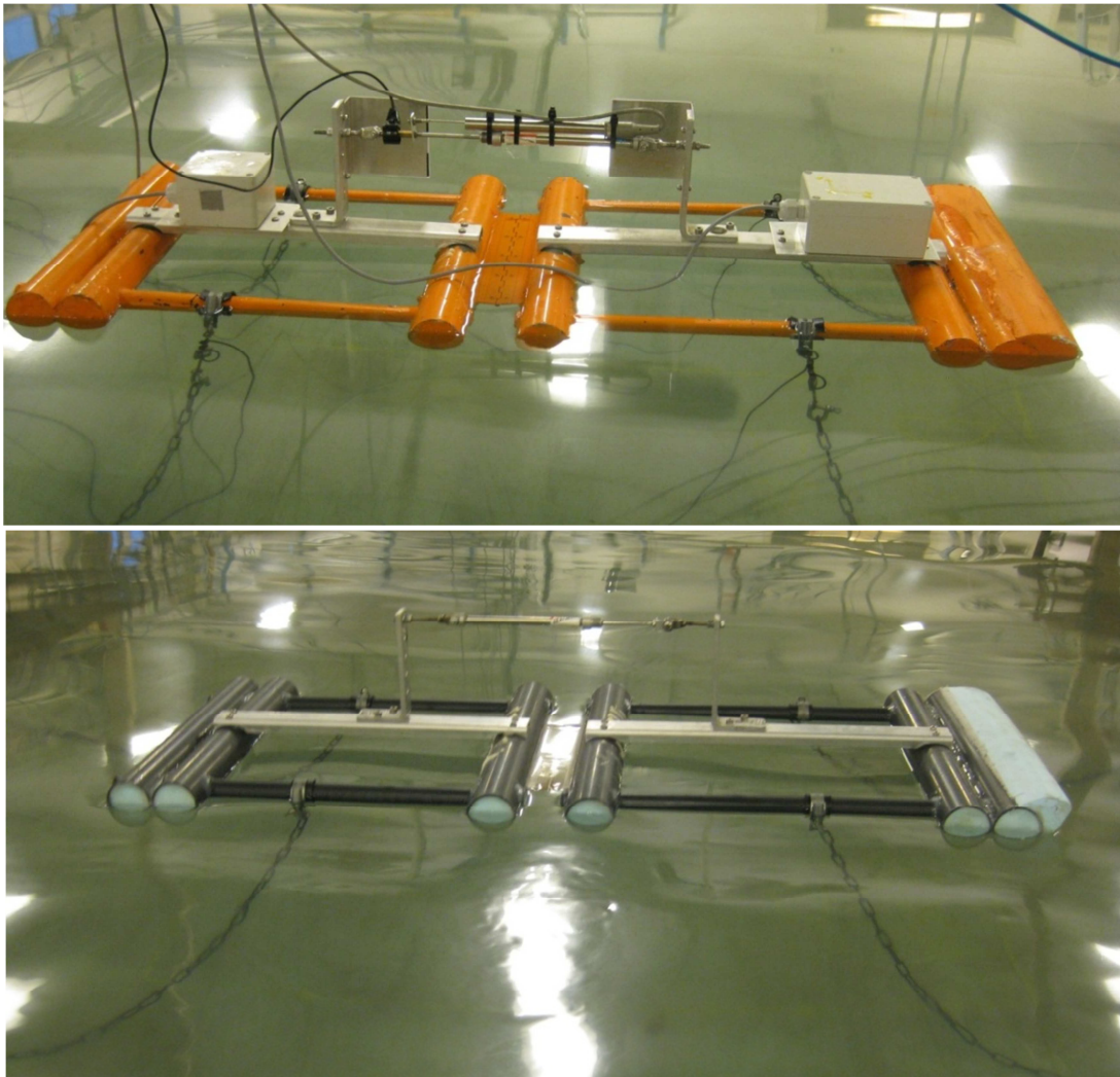
Figure 8.2 – Models of the Wave Activated Bodies with spread mooring system, in scale 1:60.
