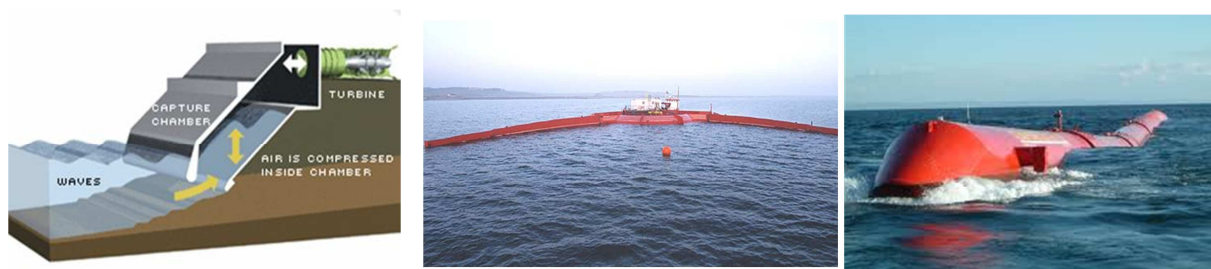
Figure 4.3 – Third classification of WECs based on the conversion principle, i.e. from the left to the right: Limpet (fixed OWC, http://www.wavegen.co.uk/what_we_offer_limpet.htm ), WaveDragon (floating OTD, http://www.wavedragon.net ) and Pelamis (near-shore WAB, http://www.pelamiswave.com )
