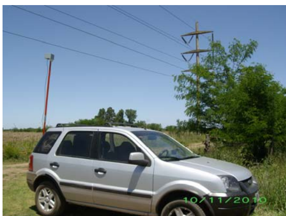
Fig. 6. EFS placement nearby an overhead line.
