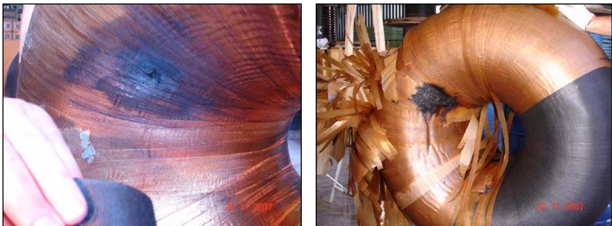
Figure 9. Metallic layer and paper affected by internal discharges.
