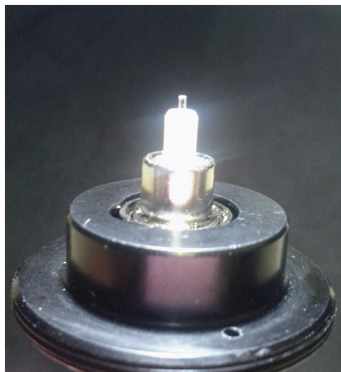
Figure 3.5: The GRIN lens ( L_4 ) bound on the optical outlet of the single mode fibre.
