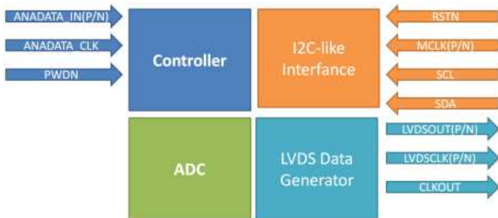
Fig. 12: Schema a blocchi del chip companion EYE-TECHDigitalOut
