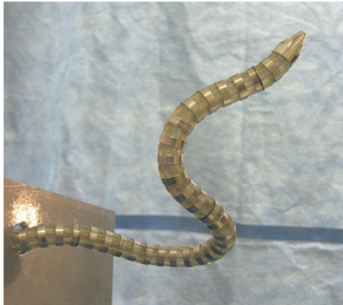
Figure 6. Distal apparatus of the CardioARM
