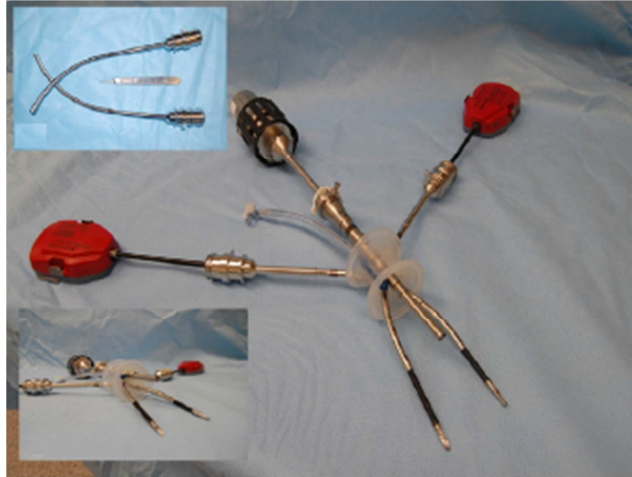
Figure 5. VeSPA instruments and accessories: curved cannulae and multichannel single-port, 8.5-mm robotic scope, flexible instruments passed through the cannulae
