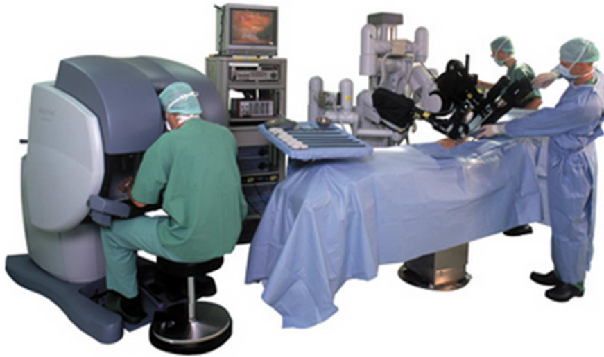
Figure 3. Overview of the Da Vinci Surgical System [7]: on the left the surgeon console is shown; on the right the patient cart with three instrument arms and the vision cart are illustrated.
