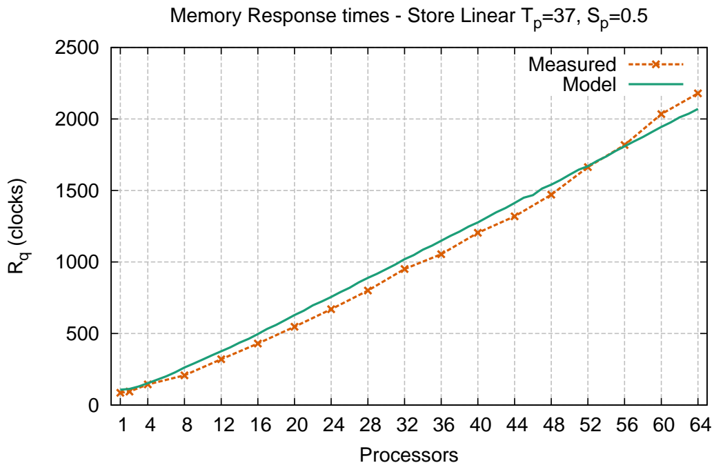
Figure 5.29: Comparison between architecture and model values of R_q for the store_linear benchmark with T_p = 37, S_p = 0.5 . Times in clock cycles.
