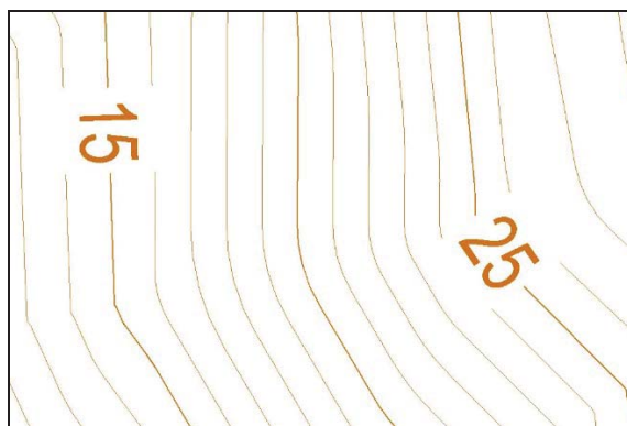
Fig. 10. An example of interrupting neighbouring contour lines in the automatic addition of a height feature.
