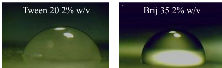
Figure 2.13: View of treated PDMS transparency loss, tolerable only in PDM-S/Brij 35 case.
