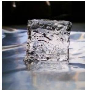
Figure 4.19: The PAAM "cube": view of the polymerised PAAM cube inside the GM;
