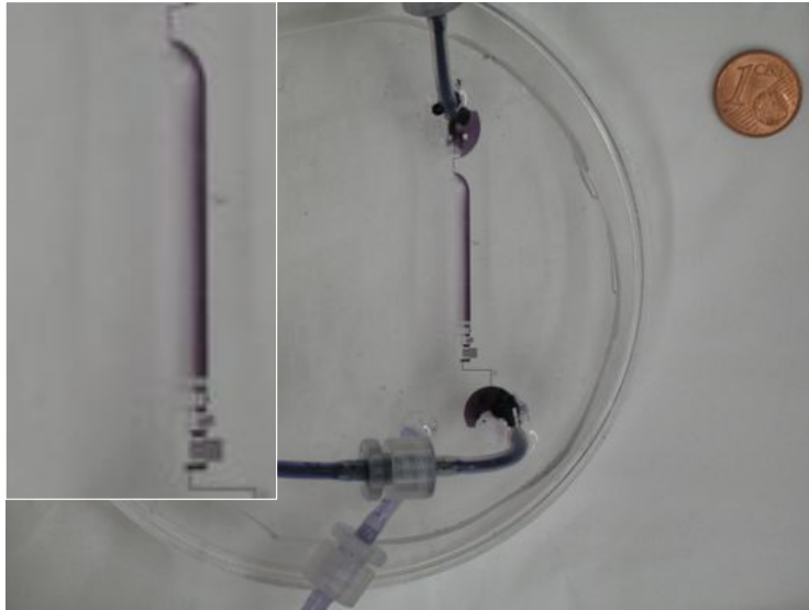
Figure 1.14: View of the Ink gradient developing within the chamber.
