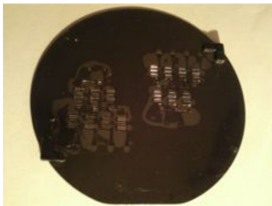
Figure 4.4: Realisation of SU-8 negative on the silicon wafer.
