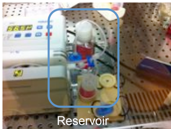
Figure 3.10: View of the two reservoirs. The larger one contains blank culture medium, while the smaller one contains a 10^{-2} mM solution of H_2O_2 in medium culture.
