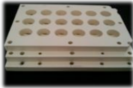
Figure 4.15: Mechanical characterisation of PAAM hydrogels in function of BIS concentration: view of the support used for uniform testing samples making;
