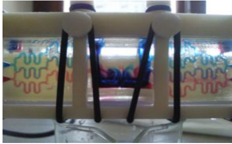
Figure 4.11: Front view of the assembled device with a dye gradient developing inside.
