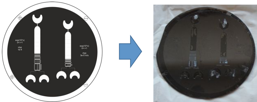
Figure 1.9: Workflow: from mask design to silicon wafer realisation.
