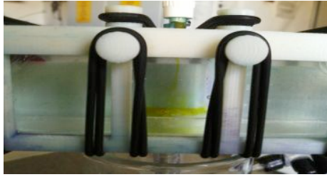
Figure 4.18: Example of catalyst infusion into the main chamber using a yellow dye.
