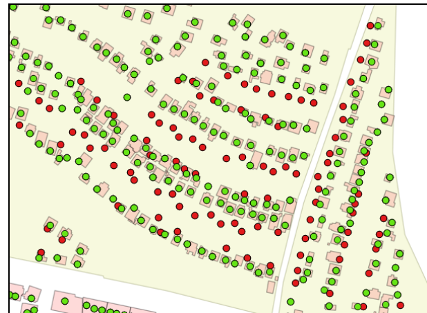
Figure 5. Example of addresses falling outside the building geometries (in red) and after editing (in green)
