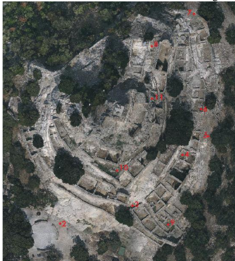
Figure 6. The eleven vertices of the topographic network superimposed to the orthophoto generated from low altitude drone flights.
