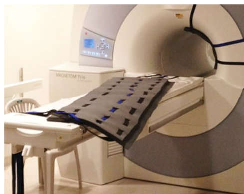
Fig. 2 MRI scanner with sound-insulating foam insert (Ultra Barrier HD Composite; American Micro Industries, Chambersburg, PA, USA) being installed into the bore of the scanner. Straps are used to hold the foam insert tight to the bore of the scanner. Noise reductions of up to 20 dB can be achieved
