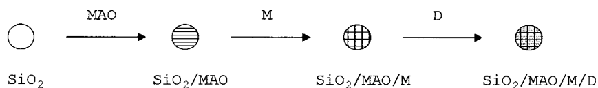
Figure 3. Preparation of labeled catalysts. M = metallocene, D = dye, MAO = methylaluminoxane.
