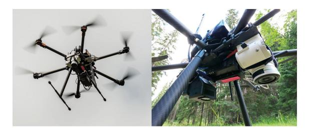
**Fig. 4.** UAV system (left) based on a Tarot 960 hexacopter and close-up of the sensor configuration (right) (Photographs by Tapio Huttunen).
