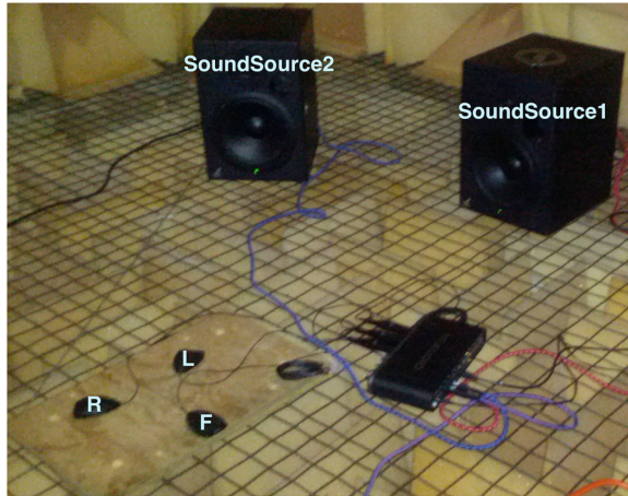
Figure 5 The anechoic chamber testing scenario of the proposed system. This scenario set in the anechoic chamber was one in which the system was tested. It shows that there are no diffracting objects inside the microphone array.
