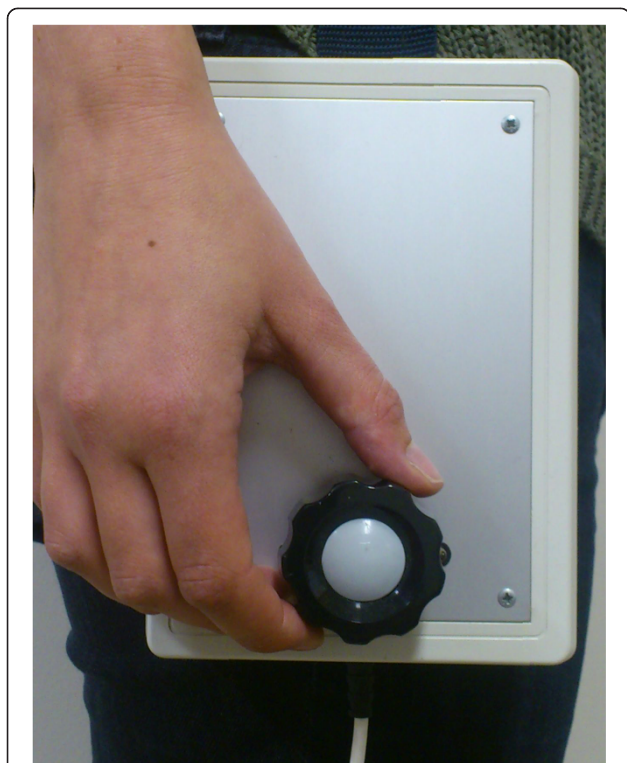
Figure 1 Custom turning knob used for recording time-varying pain throughout the entire breast compression cycle.
