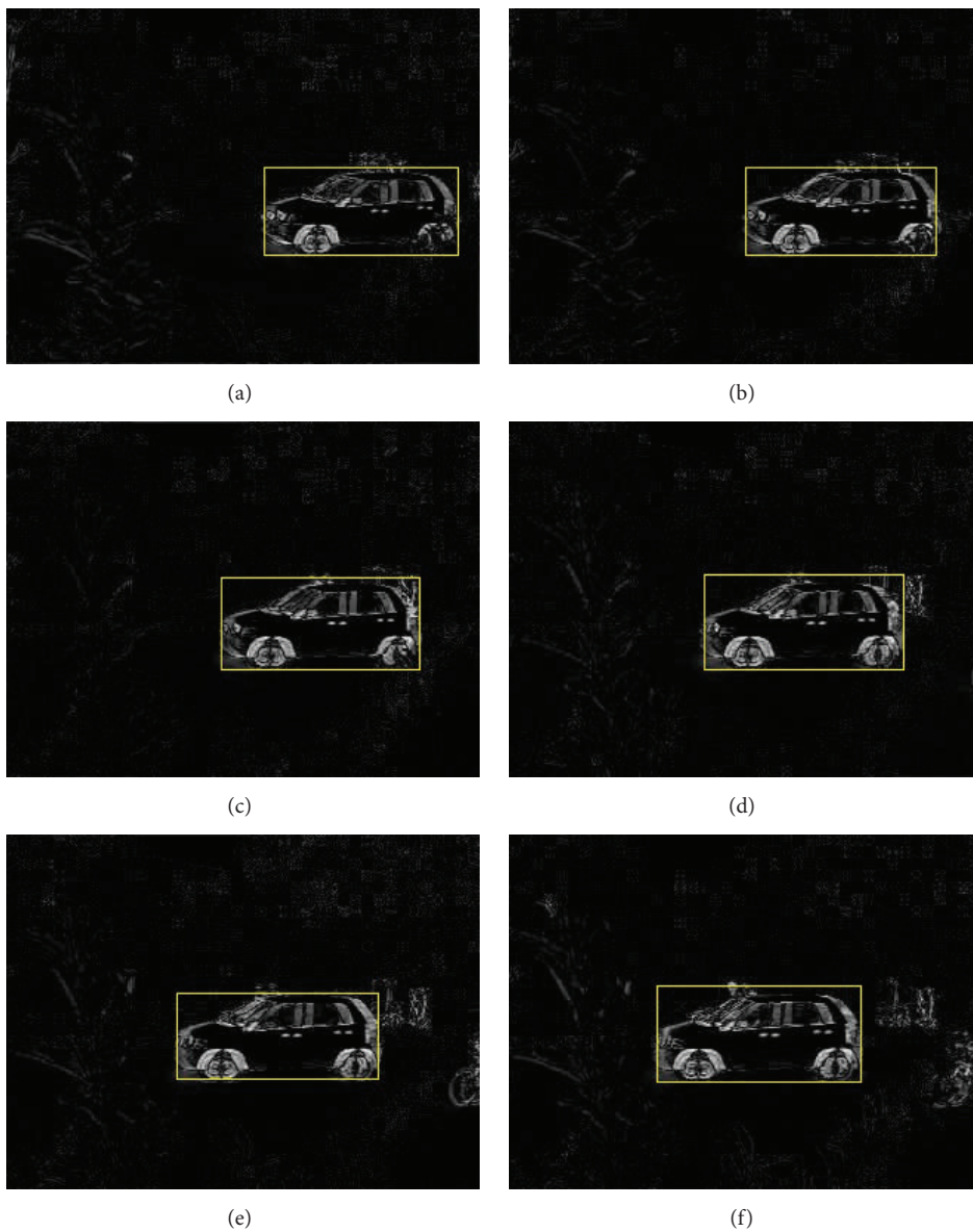
FIGURE 10: Tracking a moving car using matched corner points by FAB descriptor; DOI are showing the new location of the moving object.
