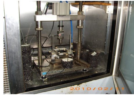
FIGURE 1: The testing machine (Universal Materials Testing Apparatus (UMATTA)) and the CR-reinforced SMA samples.
