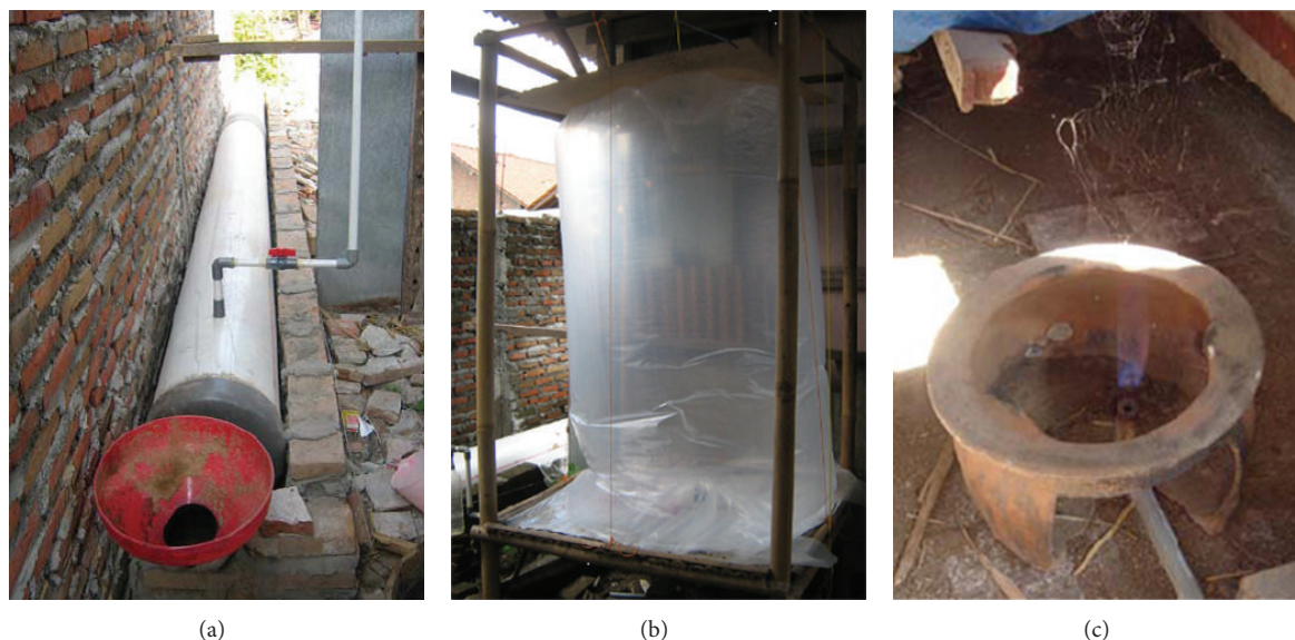
FIGURE 1: Field-scale Indonesian model digester. Pictures of a typical household biogas system: (a) the PVC digester, (b) the biogas collection bag, and (c) a traditional household cook stove fueled with biogas from the household digester.
