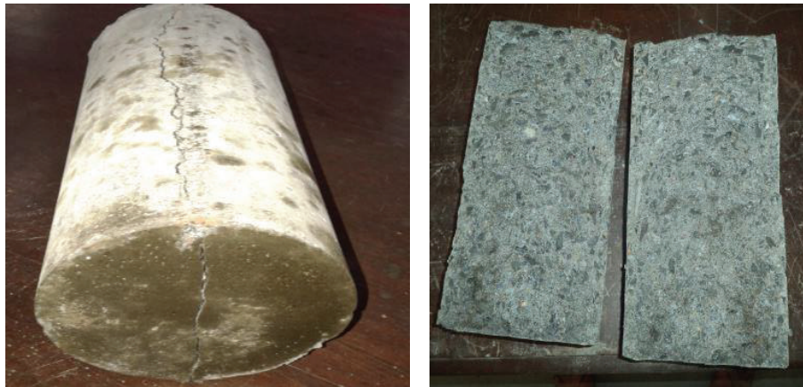
FIGURE 17: Visual of split tensile fracture.
