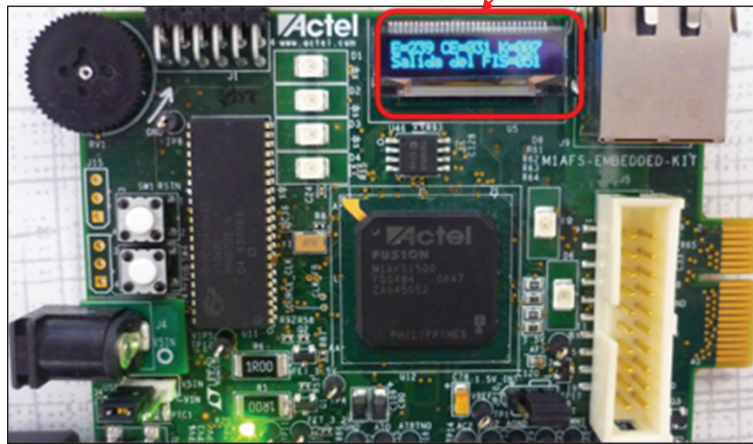
FIGURE 11: Actel development board for FPGA model “Embedded M1AFs1500 KIT”
