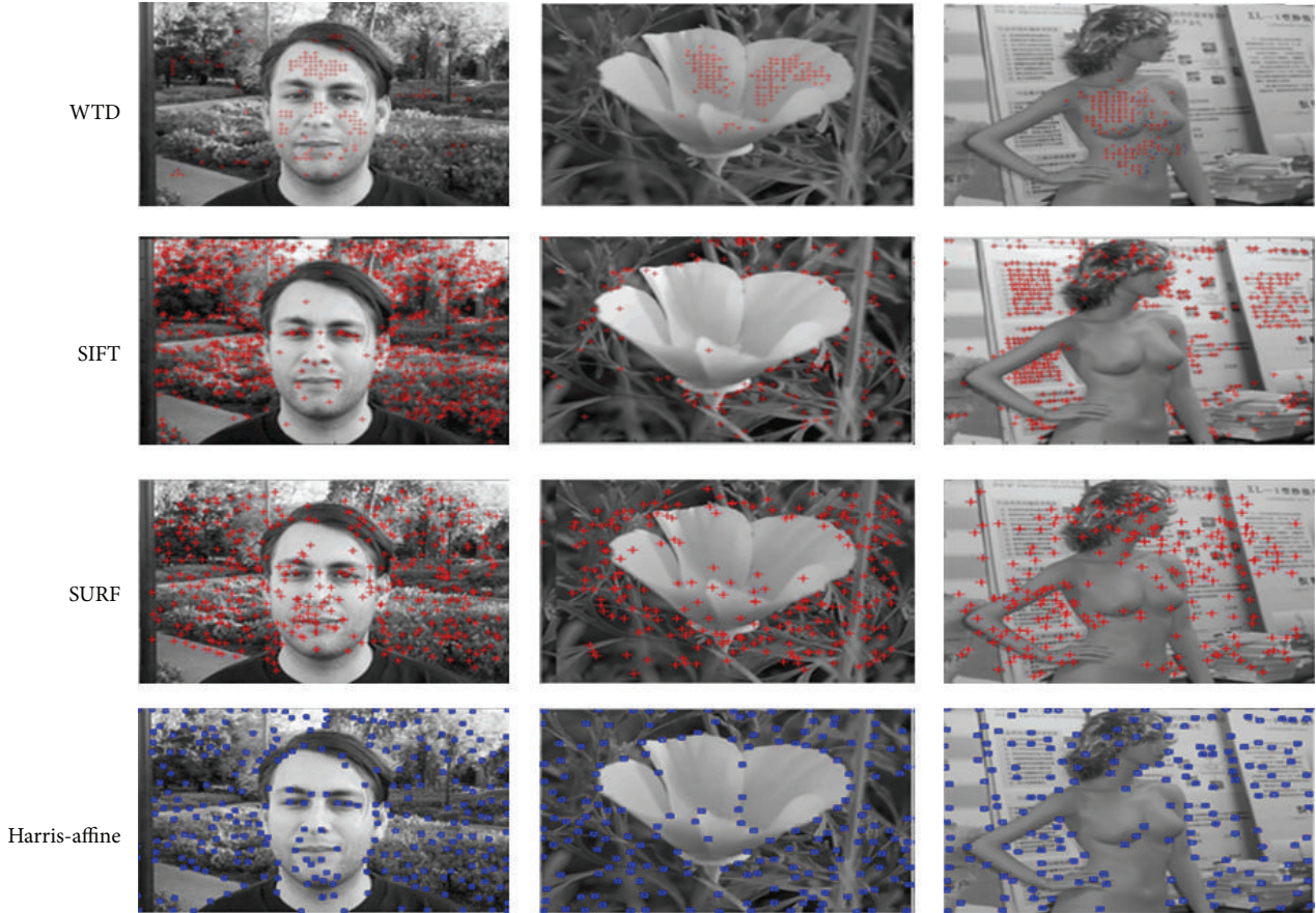
FIGURE 12: Examples of detected points distributed on different objects with different detectors.
