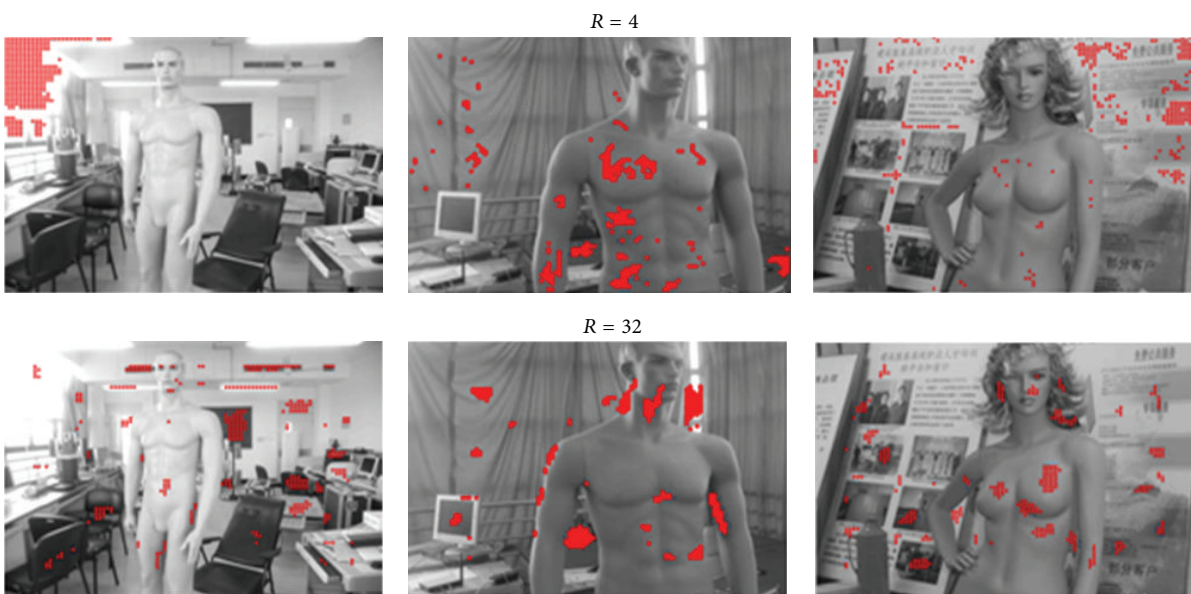
FIGURE 4: Extracted points under radii R = 4 and R = 32 .
