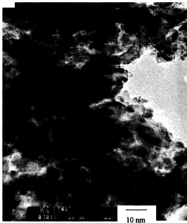
FIGURE 11. TEM micrograph of nanocrystalline ' \text{LiMn}_2\text{O}_4 '. The average crystallite size is \sim 50 Å.
