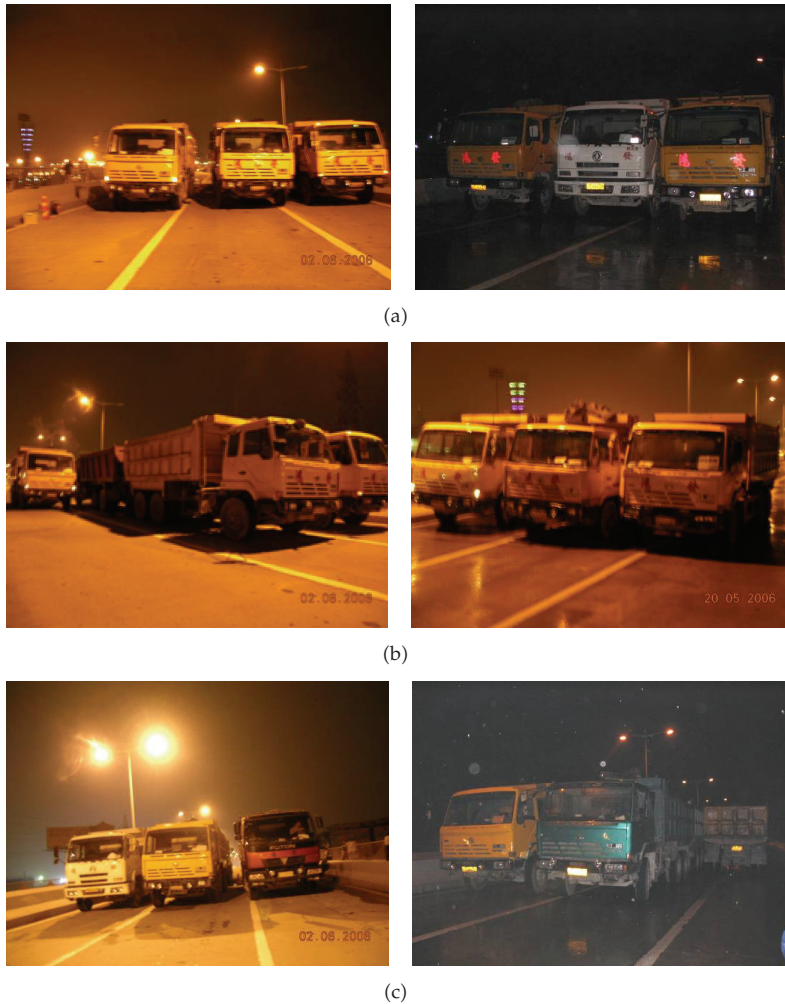
Figure 9: Photos of three critical load cases: (a) field loading on the main span (16-17#); (b) field loading on the main span (14-15#); (c) field loading on the main span (15-16#).
