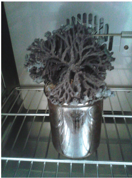
FIGURE 2: Photograph of Mn_{0.8}Zn_{0.2}Fe_2O_4 ferrite after autocombustion process.
