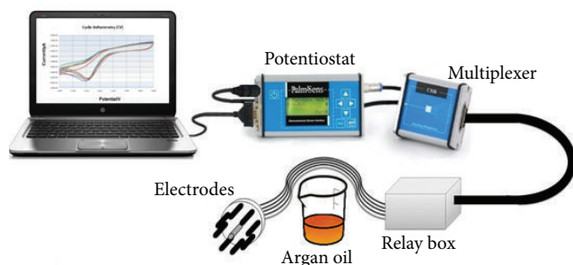
FIGURE 2: VE-tongue setup for the adulteration detection of Moroccan argan oil.
