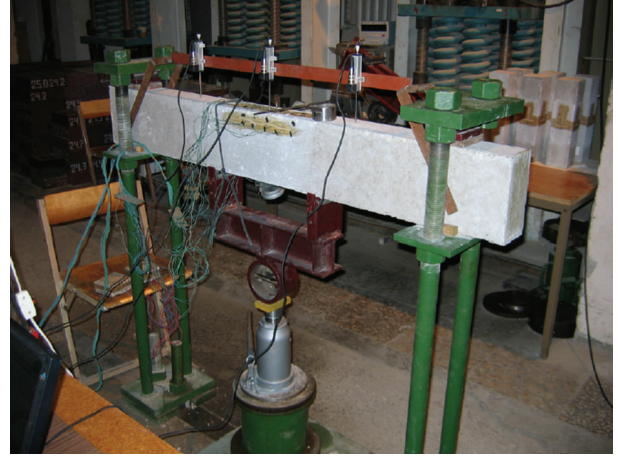
FIGURE 1: The test setup for concrete beams.
