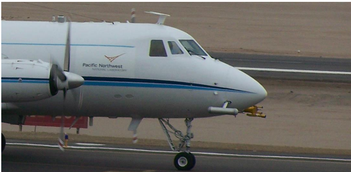
Figure 5, Showing pylon mounted PMS canisters on the nose of NCAR's Gulfstream 1 research airplane
