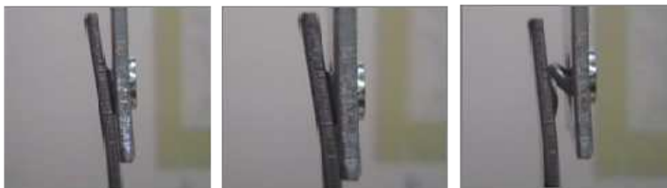
Fig. 11. Failure mode of the clinched joints
