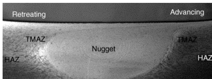
Fig. 10. Typical macrograph showing various micro-structural zones in FSP 7075Al-T651 (standard threaded pin, 400 rpm and 51 mm/min) [8].
