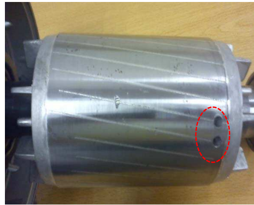
(b) Rotor with two bar breakage
