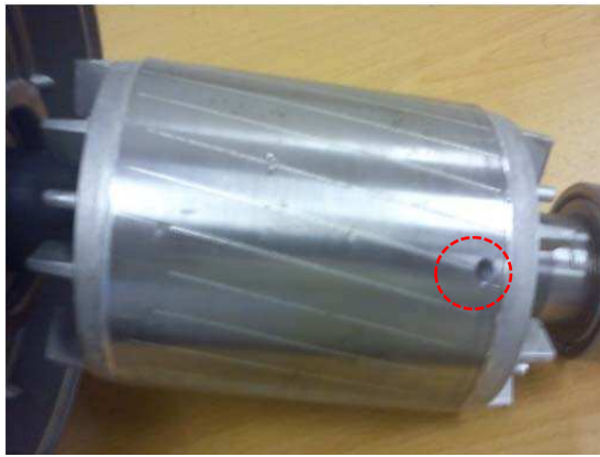
(a) Rotor with one bar breakage
